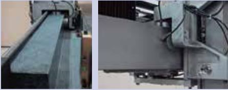
Integrated Y-Axis in Granite Table
